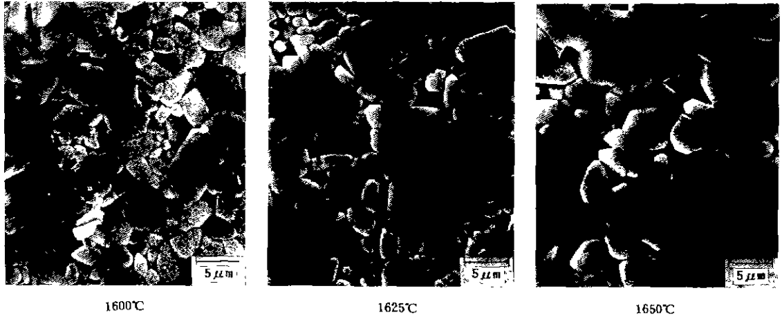
Fig. 11. Microstructures of the polished and thermally etched surfaces of alumina bodies with dopant of 0.2 wt% MgO which was sintered at various temperatures. The hydrated alumina powder was prepared by reaction of 0.125N Al_2(SO_4)_3 \cdot 16H_2O solution and 0.5 vol% NH_3/N_2 gases and then calcined at 900°C.
