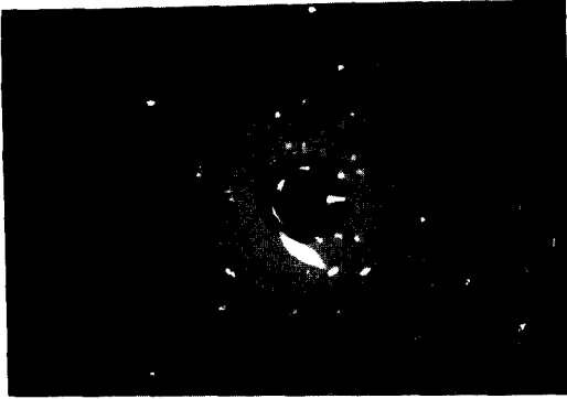
Fig. 3. Laue back reflection pattern of spodumene.
