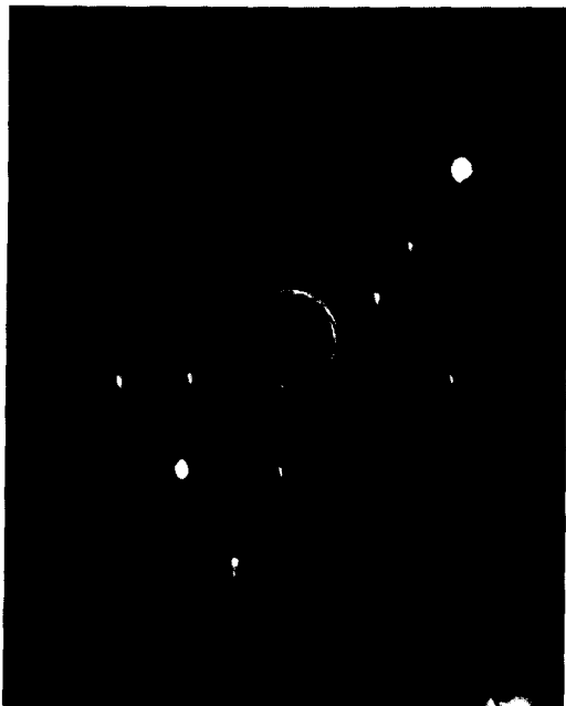
Fig. 8. Laue back reflection pattern for apatite [0001] direction in hexagonal system.
