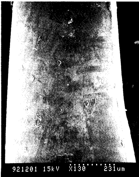
그림. 6 SEM photograph of the surface of a grown ruby fiber.
