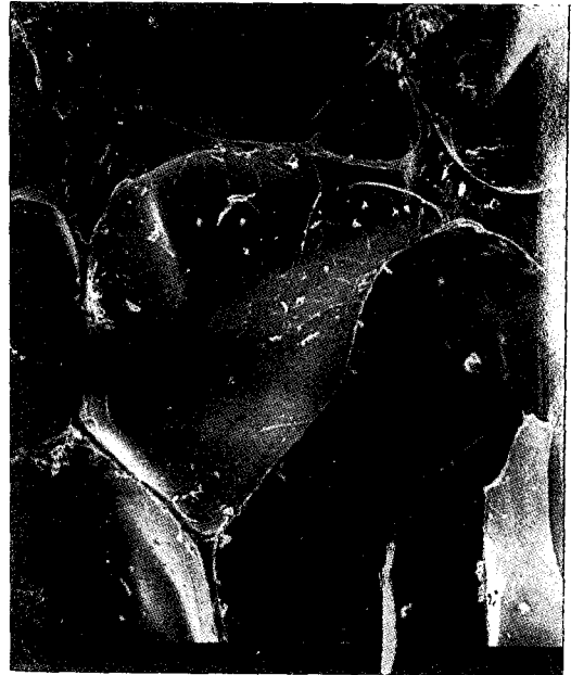
Fig. 9 Micrograph of Polyurethane Foam (density = 0.1112 g/cm 3 )
