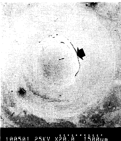
Fig. 7 SEM macro-and micro-graphs of fracture surface (loading rate : 3 \times 10^{-4} mm/min)
