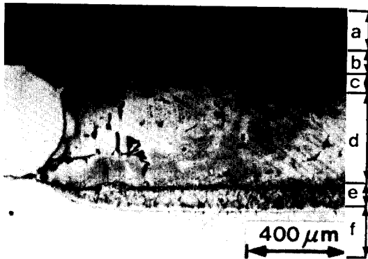
Photo. 2 Cross-sectional microstructure of Al_2O_3 /Cu-7.5wt% Zr/STS304 joint brazed at 1373K for 1.8ks (a: Al_2O_3 , b: Layer I, c: Layer II, d: Layer III, e: Layer IV, f: STS304)
