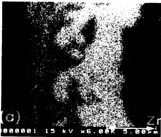
Photo. 4 SEM micrographs and X-ray image patterns for Al, Cu and Zr of the layer I and II brazed at 1323K for 0.6ks
