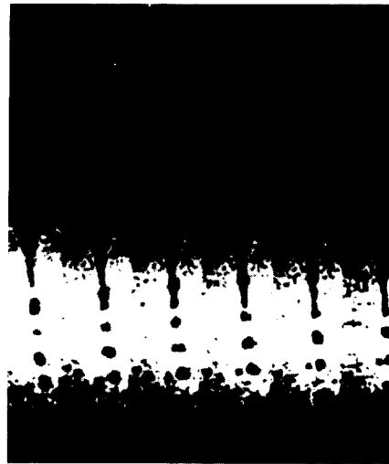
(b) Spray transfer (Shielding gas : Argon, Current : 320A Wire speed : 4.2m/min Electrode extension : 14mm)
