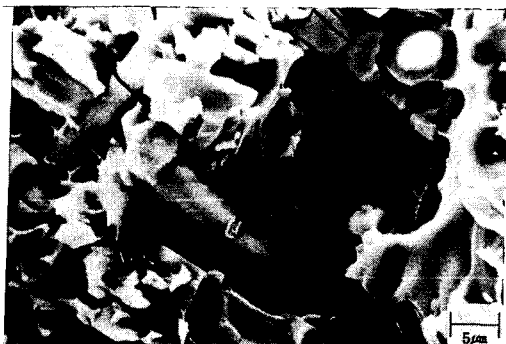
Fig. 15 SEM micrographs in the fracture surface of tensile test specimens of metal matrix composites with matrix alloy Al7075 fabricated by squeeze casting T_m=450^\circ\text{C} , T_1=800^\circ\text{C} , T_p=400^\circ\text{C} , V_f=23\% , P=75\text{ Mpa}
