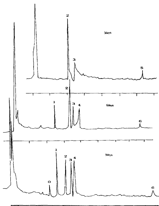
Fig. 1. GC chromatogram of oxidized TML group (peak 0: methyl octanoate, peak 1: methyl-8-(2-furyl)octanoate, peak 2: methyl linoleate, peak 3: methyl-9-hydroxy cis, trans isomer and methyl-13-hydroxy cis, trans isomer, peak 4: methyl-9-hydroxy trans, trans isomer and methyl-13-hydroxy trans, trans isomer, peak 5: α-tocopherol, peak 6: α-tocopherol quinone)
