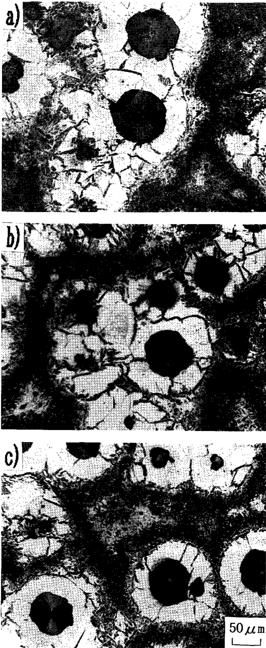
Photo 7. Microstructure of the specimens austempered at 400°C for 30min after austenitizing at 875°C for 350 sec. a) Alloy 1 b) Alloy 2 c) Alloy 3
