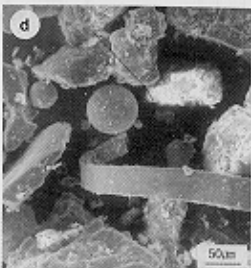
Fig 7 SEM images showing the well crystallized mineral
