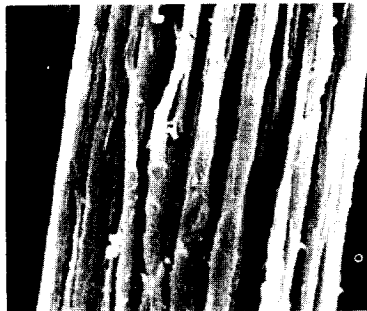
Fig. 5. Side view of micro groove fiber.
