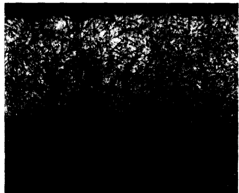
Photo 1. Optical micro structure from surface the diffusion treatment at 1123K-3.6ks after carburizing at 1233K-3.6ks in propan only( \times 100 ).
