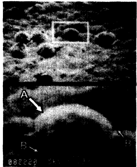
Photo 2. SEM micrographs of the surface grain structures of TiN coatings deposited on STD 61 steels. (deposition time 180 min./deposition pressure 0.5 Torr) (A) growth grain (B) death grains
