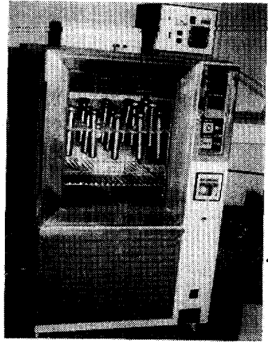
Fig. 7 Automatic cooling and heating device.
