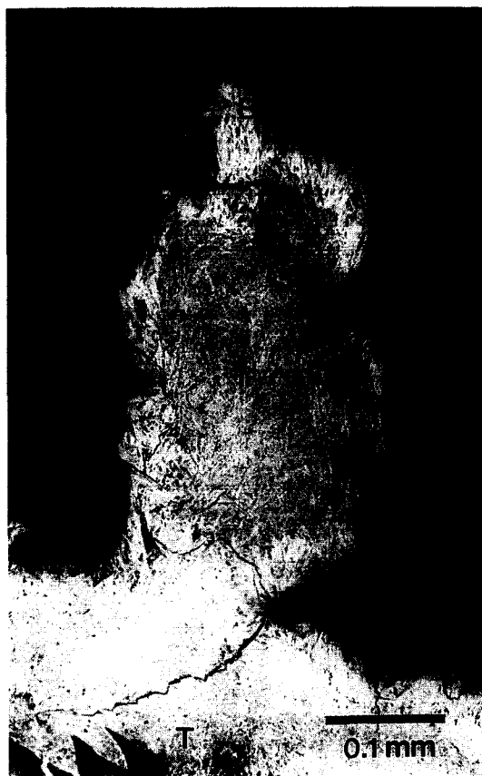
Fig. 1. Microphotograph of (Ca, Mg)-buserite-rancieite (B) and takanelite (T) from Janggun mine, Korea.
