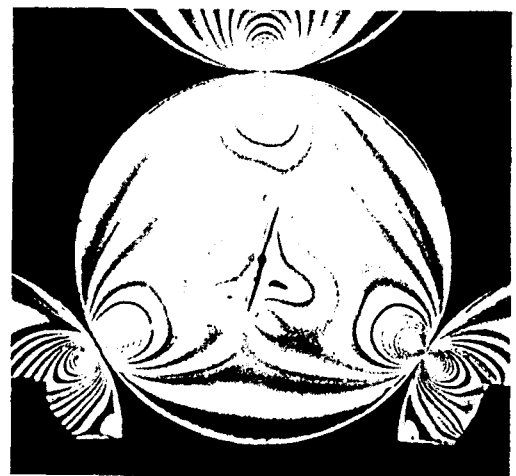
Fig. 3 Isochromatic fringe patterns of the center cracked disc specimen.
