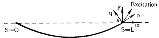
Fig.1 Excitation and lagrangian coordinates
