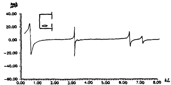
Fig.4 Heave added mass of a ship in a rectangular harbor( l_v = 1500m )
