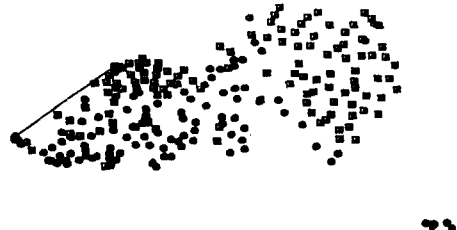
Fig. 2. Distribution of vortex varied with the passage of time around the flat otter board at \alpha=35^\circ .
