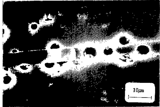
Fig. 7. Microstructures of cross-sectional view, parallel to fiber orientation, of composite burned-out in vacuum ( 10^{-6} Torr) at 400^{\circ}\text{C} for 1h and hot-pressed under 15 MPa at 1100^{\circ}\text{C} for 10 min in Ar. These show that pores are preferentially developed around carbon fiber.
