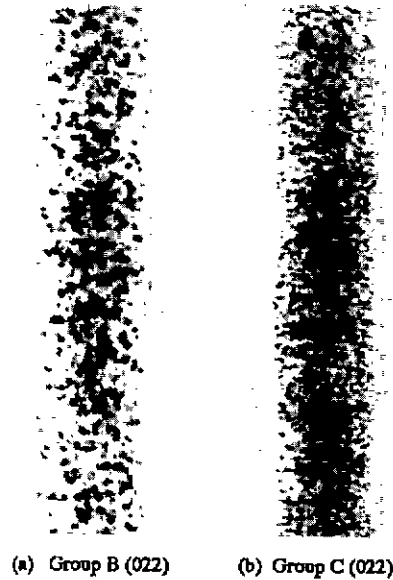
Fig. 6. Synchrotron section topographs of Group B and Group C wafers, which had been subjected to a low (at 775°C, 6 h)+high (at 1150°C, 7 h) pre-heat treatment.
