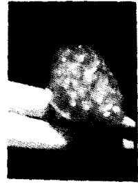
(c) pulling speed 10~12mm/h
