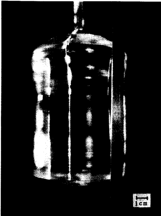
Photo 1. 128° Y LiNbO 3 single crystal grown by Czochralski technique.
