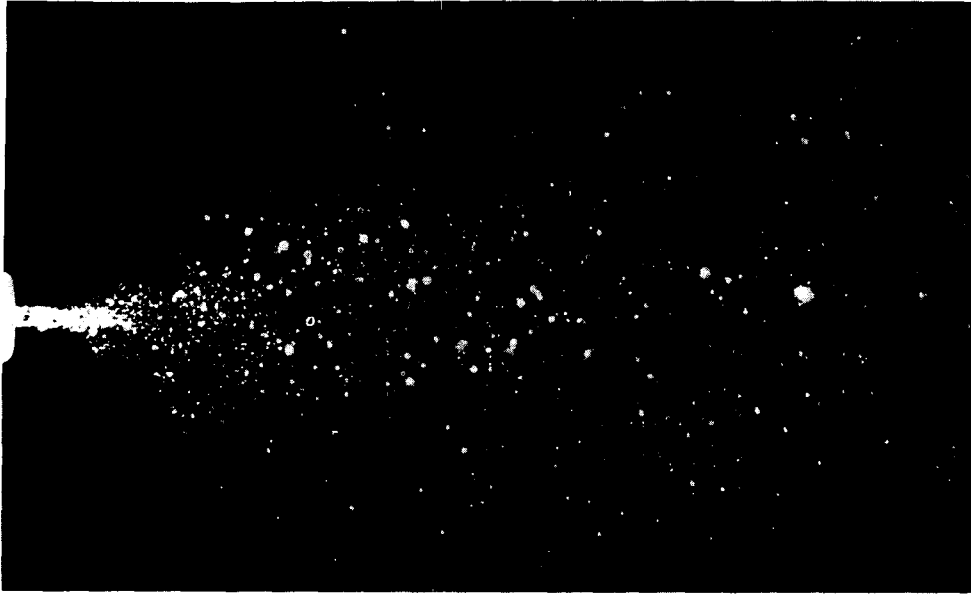
Fig. 5 Photograph of atomization for Q_{water}=0.374 ml/s, Q_{air}=81 ml/s
