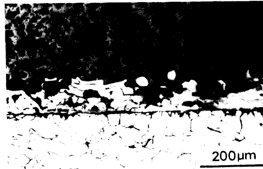
Photo. 3 Microstructure of sprayed coating after strengthening treatment at 900°C
