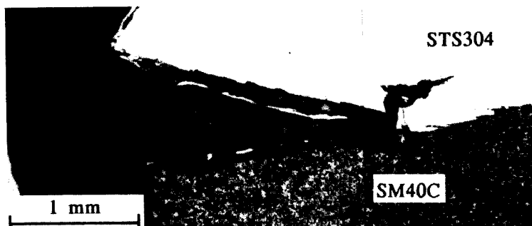
(c) initial rupture after interface fracture
