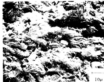
Photo. 7 EPMA results of fracture surface (Cr coating)
