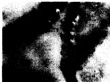
Photo.5 Poplar Cell corner, 76.8% delignified. Cooking time 160min. Bar=0.25µm.
