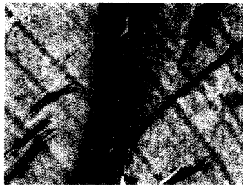
Photo.23 Korean pine Cell wall, 26.8% delignified. Cooking time 60min. Bar=0.17 \mu m.
