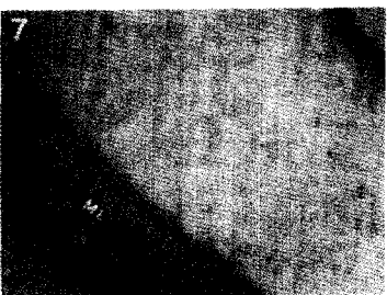
Photo.7 Poplar Cell wall, 38.5% delignified. Cooking time 20min. Bar=0.25µm.
