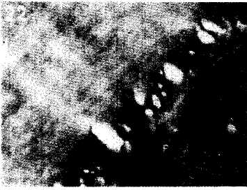
Photo.22 Korean pine Cell wall, 14.5% delignified. Cooking time 20min. Bar=0.17 \mu m.
