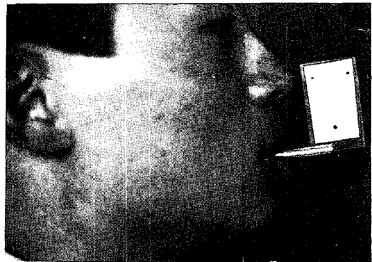
Fig. 1. Attachment of resin open clutch with three markers on plastic plate and set-up video system.
