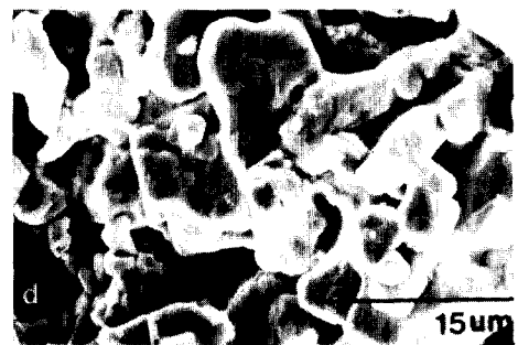
Photo. 2. SEM photographs of Y_1Ba_2Cu_3O_{7-x} . (a) calcination at 790^\circ C , (b) calcination at 900^\circ C , (c) calcination at 940^\circ C , (d) calcination at 1000^\circ C .
