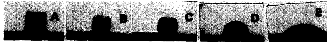
Photo 3. The change of contact angle by sealing glass(S-4) on Mn-Zn ferrite single crystal in air atmosphere A : room temp. B : 590°C C : 600°C D : 640°C E : 690°C.
