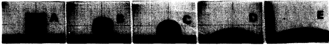
Photo 1. The change of contact angle by sealing glass (S-2) on Mn-Zn ferrite single crystal in air atmosphere A : room temp. B : 540°C C : 570°C D : 600°C E : 640°C.
