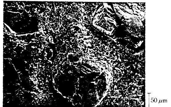
(b) After dressing Dresser : C220G8 V d = 16m/min V g = 7.85m/s h d = 20 μm T = 200sec
