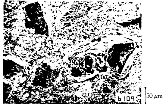
(a) After grinding Work : Si 3 N 4 V w = 20mm/min V g = 23.6m/s h = 1mm
