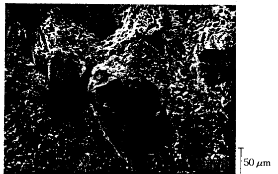
(c) After dressing Dresser : C220G8 V d = 16m/min V g = 7.85m/s h d = 20 μm T = 650sec
