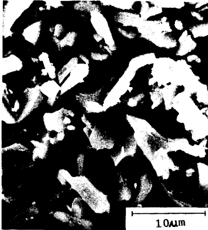
Fig. 1. Scanning electron micrograph of ferroxplana powder.
