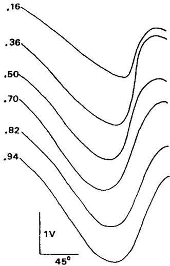
Fig. 4. The torque curves of a pure Ni wire for calibration. The values at the left of the curves represent the field intensity in tesla (Fig.5~Fig.8).
