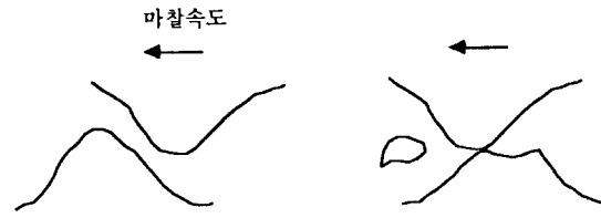
Fig. 6. Brittle fracture of asperity during friction
