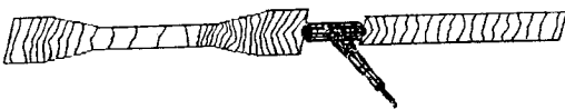
Fig. 8. Melt front advancement of the ceramic mixture injection molded using gate II.
