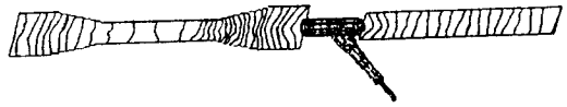
Fig. 10. Melt front advancement of the ceramic mixture injection molded using gate III.
