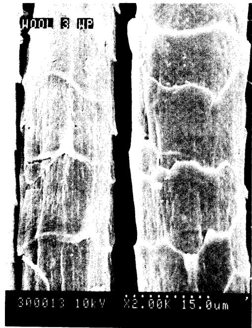
Photo. 3. Scanning electron micrograph of the surface of wool treated with Esperase 8.0L to a weight loss of 5%.
