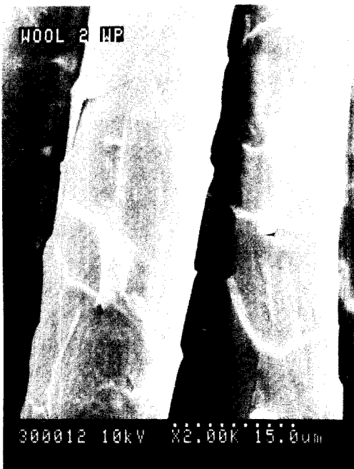
Photo. 2. Scanning electron micrograph of the surface of wool treated with Esperase 8.0L to a weight loss of 3%.
