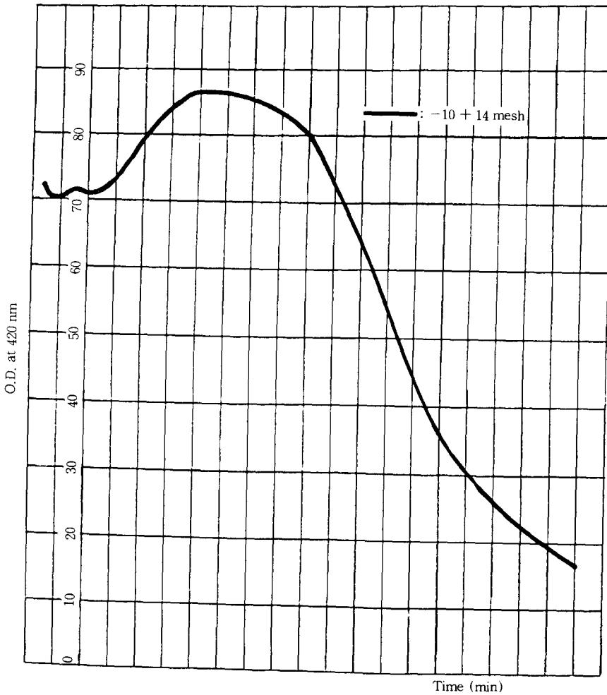
Fig. 4. Extraction curve of barley tea in packed column
