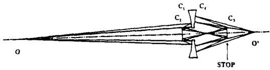
Fig. 4. Configuration of the scaled-up four-spherical mirror system. The stop of the system lies at the third mirror surface ( f' = -10 cm).
