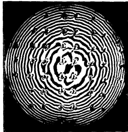
(d-2) Negative oblique slicing method Fiber dia.=0.25mm, Fitch=5mm, l=160\text{mm} Fiber direction=axis, d=40\text{mm} M_x=2.695\text{N.m} (d) Orthotropic circular shaft
