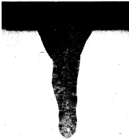
Fig. 6 Macrosection of laser weld in AISI 316 steel (Laser power, 2kW, travel speed, 3.0m/min, x25)
