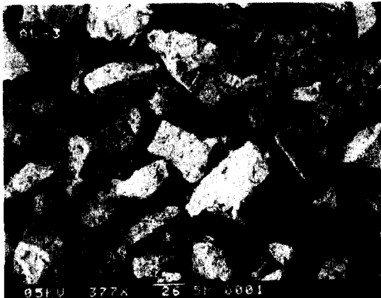
Fig. 6—SEM of hydrous aluminum oxide powder aged at 70°C for 18 hours.
