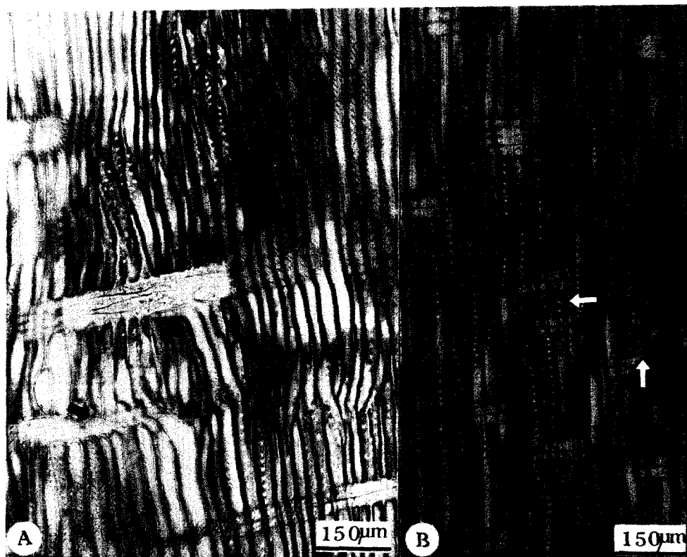
Fig.4. Radial surfaces of compression wood(A) and opposite wood(B). Arrow indicates tracheid tip distortion.
