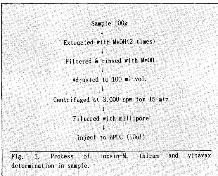
Fig. 1. Process of topsin-M, thiram and vitavax determination in sample.
