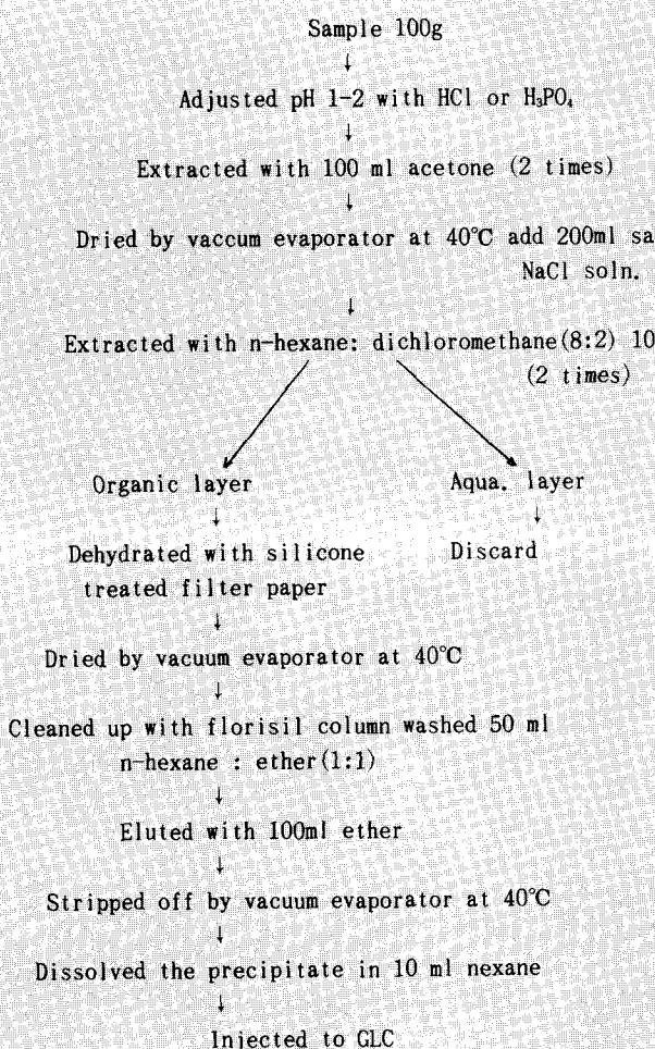
Fig. 2. Process of captan determination in sample.
