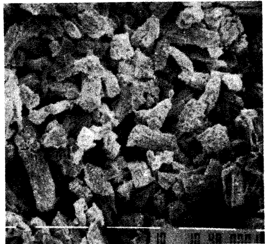
Fig. 6. SEM picture of DiNi 5 after several absorption and desorption(X 2000).
