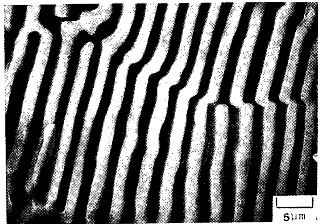
Fig. 6 Scanning electron micrograph of Al-Al 3 Ni eutectic composite.
