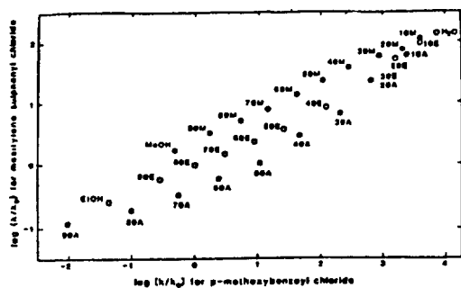
Fig. 1. Correlation of logarithms of rate constants for solvolyses of mesitylenesulphonyl chloride (1) vs. logarithms of rate constants for solvolyses of p -methoxybenzoyl chloride (3) at 25 °C; solvent codes: A = % v/v acetone/water, E = % v/v ethanol/water, M = % v/v methanol/water.
