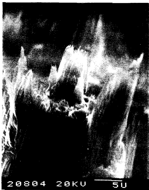
Fig. 6. SEM of Fracture specimen of 6BPAB molded at 280°C.(×3000)
